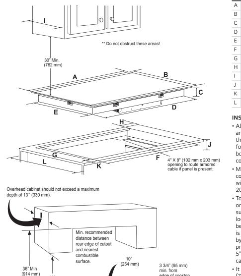
30 27/32" (783 mm) 21 15/32" (545 mm) 3 3/4" (95 mm) D 28 13/16" (732 mm) E 19 5/8" (498 mm) F 29 3/8" Minimum (746 mm) G 20 1/4" Minimum (515 mm) H 13/16" (20 mm) 13" Maximum (330 mm) 5 23/32" Minimum (145 mm) 2 1/2" (64 mm)
